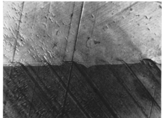
Figure 5 Bicrystal tested at 125^\circ\text{C} showing grain-boundary cracking on surface C and subsequent grain-boundary migration ( \times 440 ).
